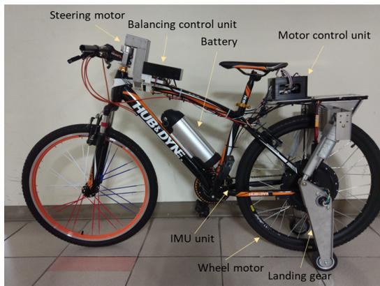
Figure 5: Photo of the prototype bicycle.
