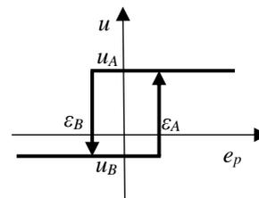
Figure 4: The static characteristic of an asymmetrical relay with hysteresis.
