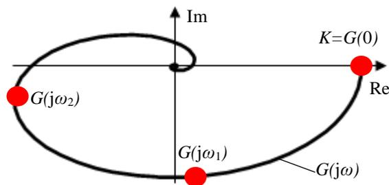
Figure 7: The Nyquist frequency characteristic of a process and the found points  $G(0)$ ,  $G(j\omega_1)$  and  $G(j\omega_2)$ .
