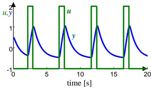
Figure 12: The time courses of the relay output  $u$  and the process output  $y$  obtained from the relay feedback experiment with integrator under the static load disturbance.
