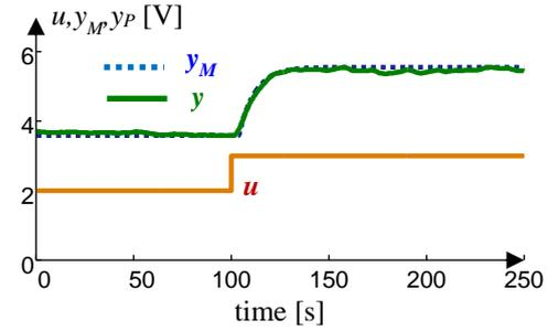
Figure 18: The time courses of the manipulated variable  $u$ , the model output  $y_M$  and the process output  $y$ .
