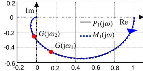
Figure 9: The Nyquist diagram for the transfer functions  $P_1(s), M_1(s)$  and the calculated points  $G(j\omega_1)$  and  $G(j\omega_2)$ .
