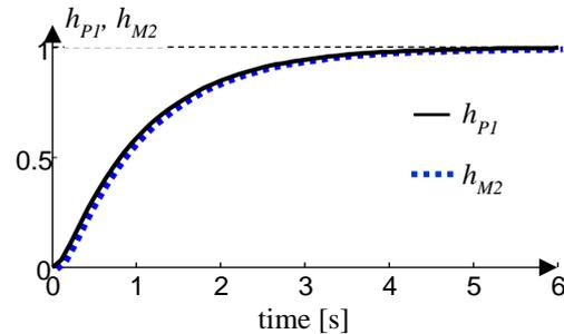
Figure 14: The step response  $h_{P1}$  of the process  $P_1$  and the step response  $h_{M2}$  of the model  $M_2$ .
