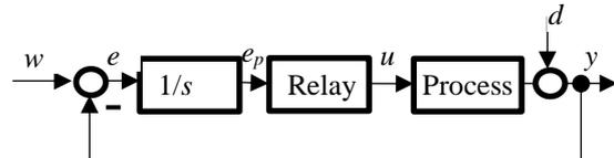
Figure 11: The process under the load disturbance  $d$  controlled by the asymmetrical relay with integrator.
