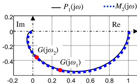
Figure 13: The Nyquist diagram for the transfer functions  $P_1(s)$ ,  $M_2(s)$  and the calculated points  $G(j\omega_1)$  and  $G(j\omega_2)$ .
