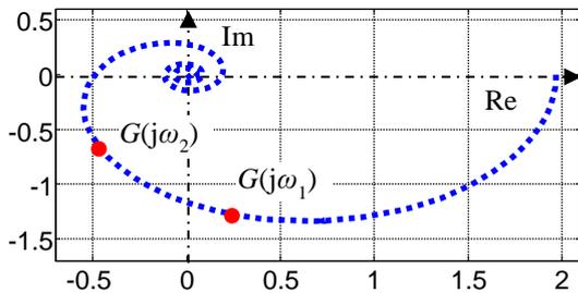
Figure 17: The Nyquist diagram for the transfer functions  $M_T(s)$  and the calculated points  $G(j\omega_1)$  and  $G(j\omega_2)$ .
