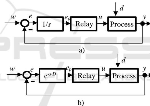
Figure 3: Block diagram of a process under relay feedback with a) integrator b) delay  $D$ .
