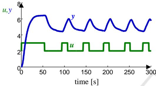
Figure 16: The time courses of the relay output  $u$  and the process output  $y$  obtained from the relay feedback experiment with integrator.
