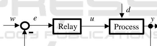
Figure 1: Block diagram of a process under relay feedback.
