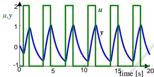
Figure 8: The time courses of the relay output  $u$  and the process output  $y$  obtained from the relay feedback experiment with integrator.
