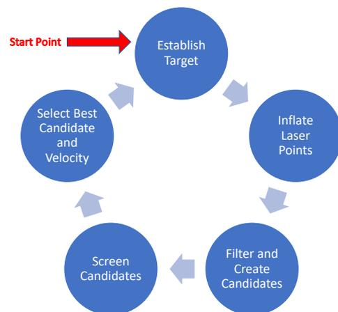
Figure 8: VFH algorithm loop.
