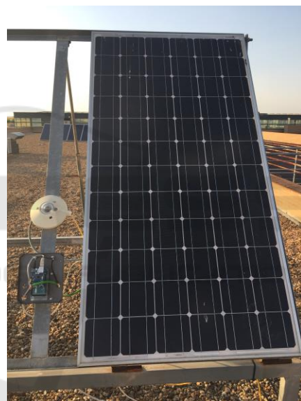
Figure 8: Experimental setup of the Arduino and the photovoltaic module.
