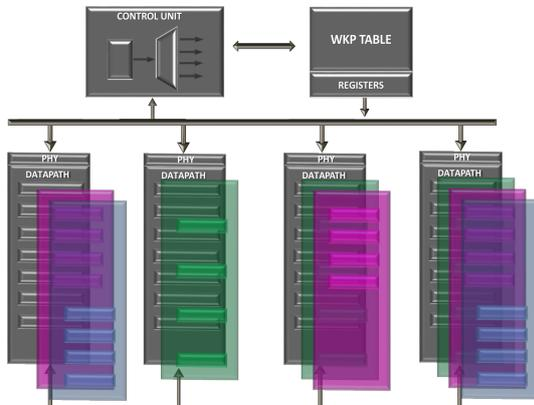
Figure 5: ETArch Switch - Virtual Datapaths.
