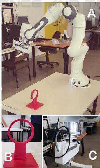
Figure 8: The robot task configuration (A). The robot's gripper is holding a hook (B) which it uses to pick up the object (C).
