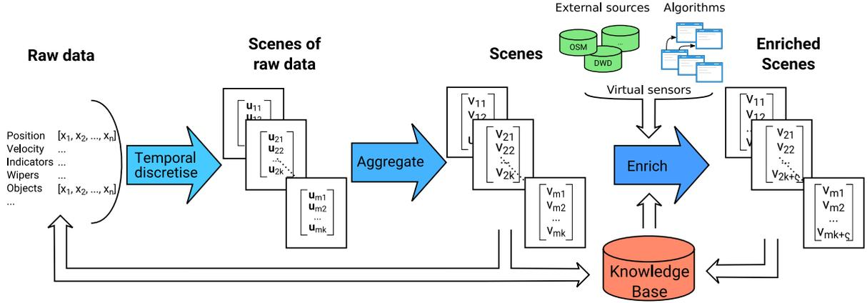
Figure 1: Three stage process for transforming the vehicle sensor data to a series of scenes enriched with additional information from algorithms and external data sources as the foundation for scene-based scenario identification.
