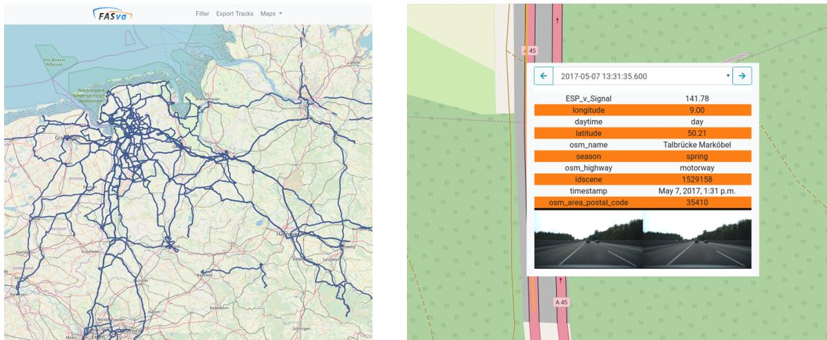
Figure 4: The *drive visualisation* service provides an interactive web-interface of the conducted test drives including filter capabilities for efficient sequence identification and track selection for scene analysis. *Left*: A map of all conducted test drives. *Right*: The same zoomed-in map showing information of a selected scene.
