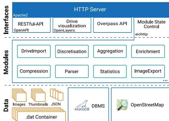
Figure 3: The architecture of the proposed VDMS for managing large-scale test campaigns consists of three layers: *Data*, *Modules* and *Interfaces*.
