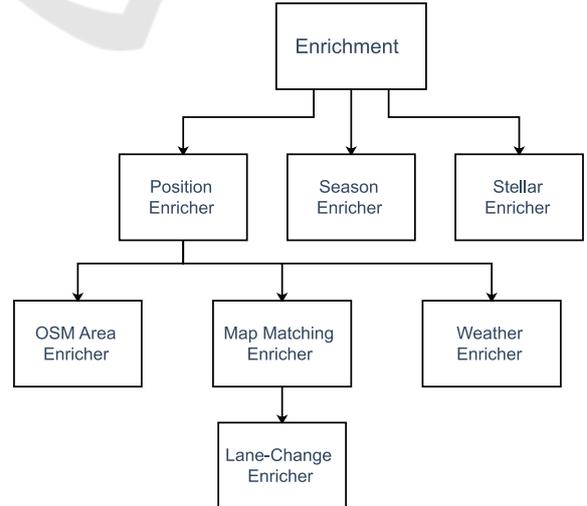
Figure 2: The enrichment module uses an acyclic graph to manage components and their dependencies for scene enrichment visualized as a tree of components.
