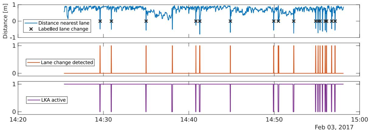
Figure 5: Sequence of a trip on a motorway with two to three lanes for demonstrating the proof-of-concept of the proposed VDMS for scenario identification and system evaluation. *Top*: Distance to nearest line and the manually labelled lane changes. *Middle*: The detected lane changes of the algorithm. *Bottom*: The signal of the onboard Lane Keep Assist System.
