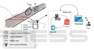
Figure 1: Architecture of bicycle counting system's prototype.
