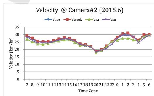
(B) Time Zone based Vehicle speed at Camera#2.
