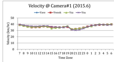
(B) Time Zone based Vehicle speed at Camera#1.
