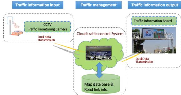
Figure 1: Traffic Management System Configuration.
