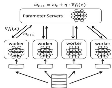
Figure 1: Data parallelism using parameter servers to exchange gradients.
