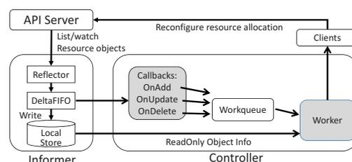
Figure 4: The interaction between a custom controller and K8S. The two gray boxes are the controller-specific components that were re-implemented in our approach.
