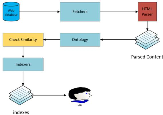
Figure 4: Crawling algorithm architecture.
