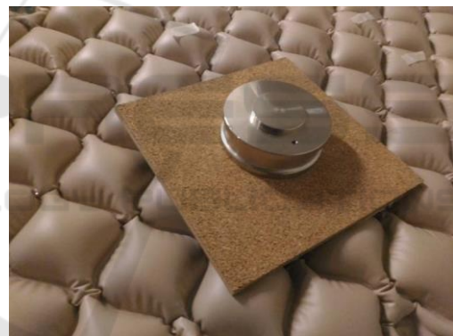
Figure 10: Calibrated weight of 10 kg placed on the air cells of the dynamic mattress.
