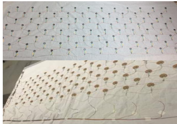
Figure 13: Sensing matrix (12x8) from commercial pressure sensors of Interlink Electronics.
