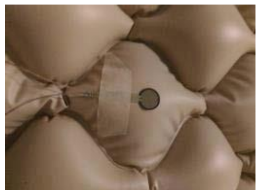
Figure 11: FSR sensor fixed to an air cell of the mattress.
