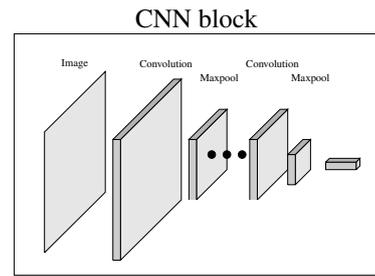
Figure 3: The structure of the CNN block.
