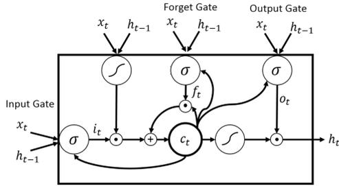
Figure 6: LSTM cell diagram from (Jain et al., 2016).
