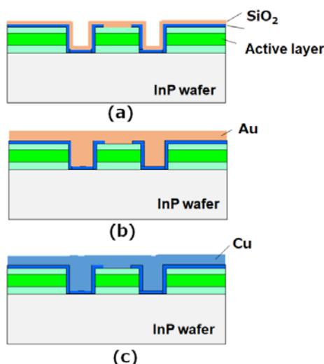
Figure 1: Devices structures. (a) Ridge covered with thin SiO<sub>2</sub> and thin Ti/Au, (b) Ridge embedded with Au, and (c) Ridge embedded with Cu.
