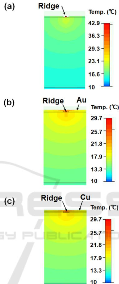
Figure 6: Simulation results. (A) Ridge covered with  $\text{SiO}_2$  and thin Ti/Cu, (B) Ridge embedded with Au and (C) Ridge embedded with Cu.
