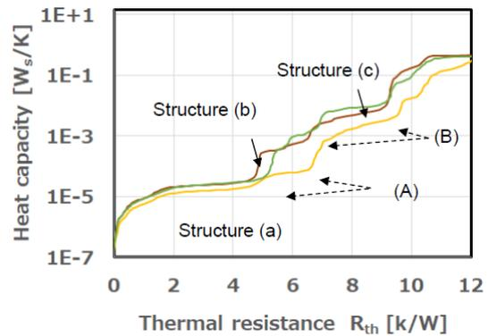
Figure 8: Thermal resistance vs. Heat capacity (Structure function).
