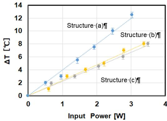
Figure 4: Temperature difference  $\Delta T$  between the ridge bottom and the bottom of the wafer (Experiment).
