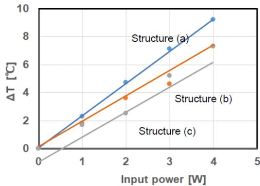
Figure 7: Temperature difference between the ridge bottom and the bottom of the wafer (Simulation).
