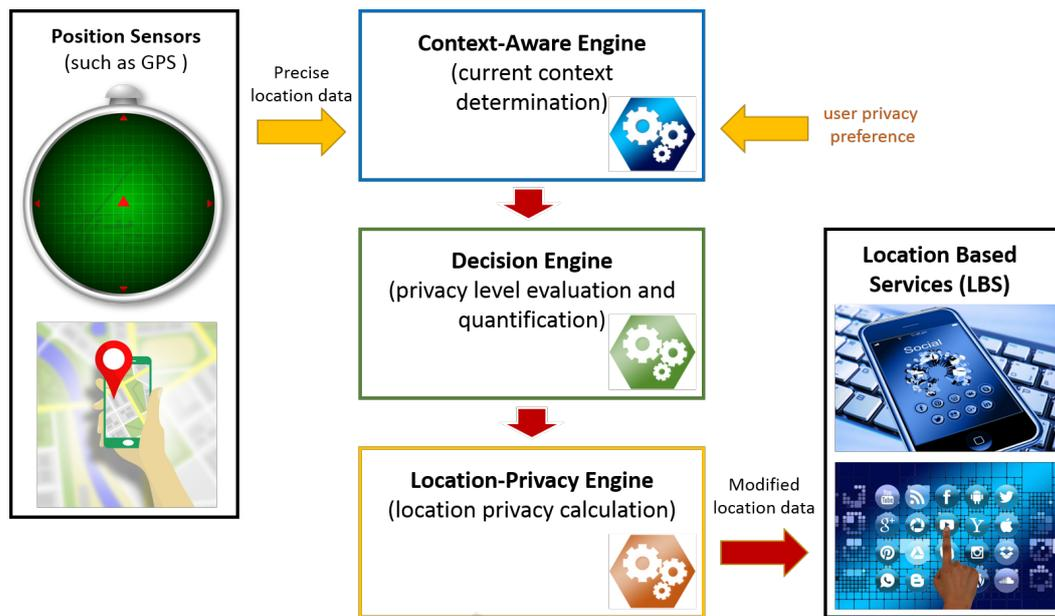
Figure 3: Proposed system architecture for Location-Privacy Assured IoT (LPA-IoT) Scheme.
