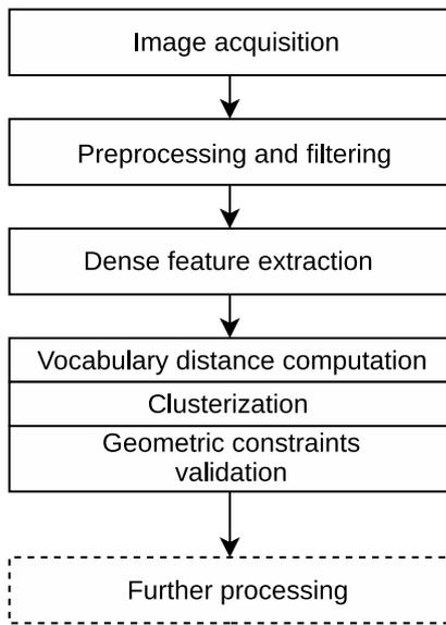
Figure 1: Eye detection system architecture.
