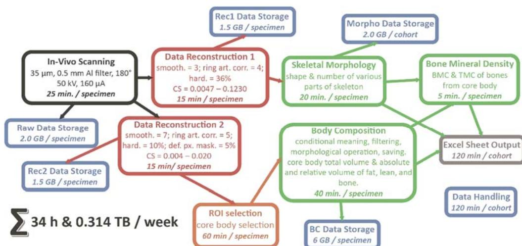
Figure 1: Scheme of adult mouse morphology and body composition workflow. Black: data acquisition; Red: data reconstruction; Orange: data preparation; Green: analysis; Blue: data storage; Grey: Excel output. smooth. = smoothing; ring art. corr. = ring artifact correction; hard. = beam hardening; def. px. mask = defect pixel masking; CS = border intensities for reconstruction.
