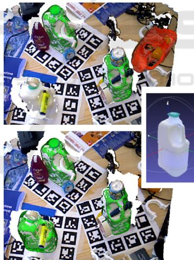
Figure 1: Multi-instance pose estimation example for a scene from the dataset of (Tejani et al., 2014). To the top is shown an example with non-optimized feature parameters, resulting in two correct (green) and one incorrect detection (red). The CAD model of the object is shown in the middle. Our parameter optimization improves the pose estimation algorithm, giving correct detection of all the three instances of the object shown at the bottom.
