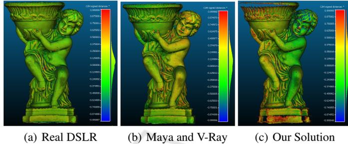
Figure 5: Heat map of the distances between the ground truth object and the reconstruction. Green indicates that the two coincide, while red and blue indicate larger positive and negative distances between the two.
