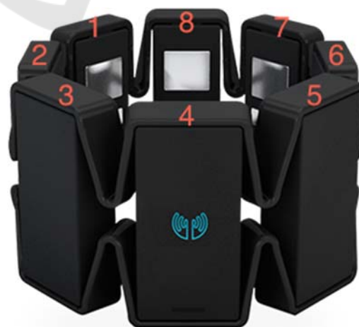
Figure 3: Myo armband - EMG sensors numbered from 1 to 8.
