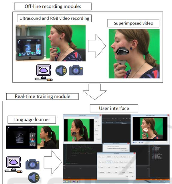
Figure 2: Schematic of our language training system. Language learner can see both off-line and real-time data on a computer screen. The off-line video is played with a small delay and language learner imitate that word. The learner comprehends the differences between two videos and tries to duplicate instructor's video.
