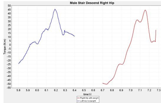
Figure 18: Hip Extension/Flexion torque values for the stair descend trials with the male subject.
