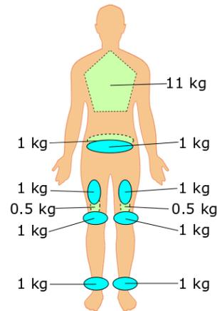
Figure 4: Distribution of the attached weights to approach the weight dynamics of the exoskeleton developed.
