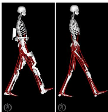
Figure 11: Screenshot of the simulation with the male model with the exoskeleton on the left and without the exoskeleton on the right.
