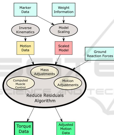
Figure 9: Workflow for the OpenSim Simulation Toolkit to achieve precise values for joint torques using RRA.
