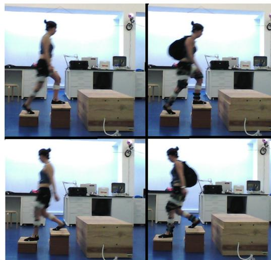
Figure 8: Pictures of the female subject performing stair trials with normal clothing on the left and attached weights on the right. The top two pictures show stair climbing while the bottom pictures show stair descending.
