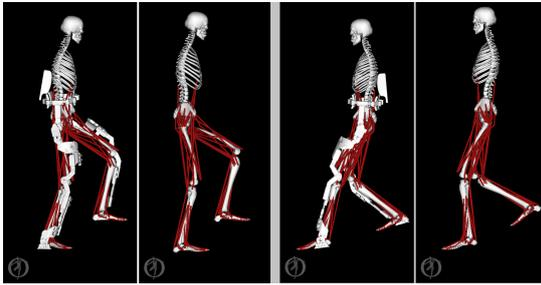
Figure 15: Screenshot of the simulation with the male model with and without the exoskeleton while climbing stairs on the left and descending stairs on the right.
