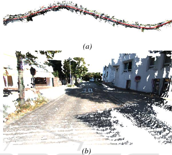
Figure 13: 3D dense reconstruction based on the KITTI dataset. (a) Full 3D dense point cloud generated using the KITTI dataset. The red points show the trajectory computed by our adaptive SLAM. (b) Zoom inside the point cloud. Here, several depth maps have been merged to create a unique cloud.
