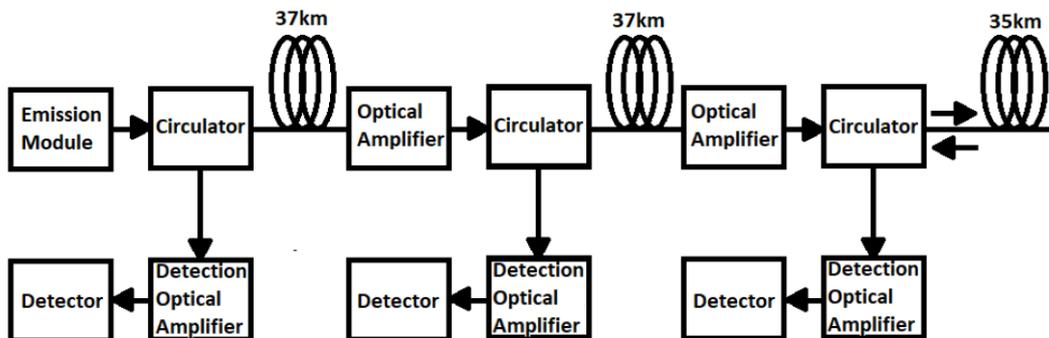
Figure 2: Experimental setup. Direct-detecting  $\Phi$ -OTDR system with the addition of the distributed sensing system.
