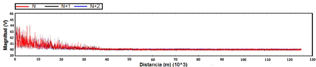
Figure 4: Detected interferences in a trace along the length (109km) of the three coils in a single phase.
