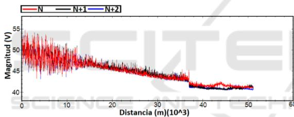
Figure 6: MI-induced fading in a trace.
