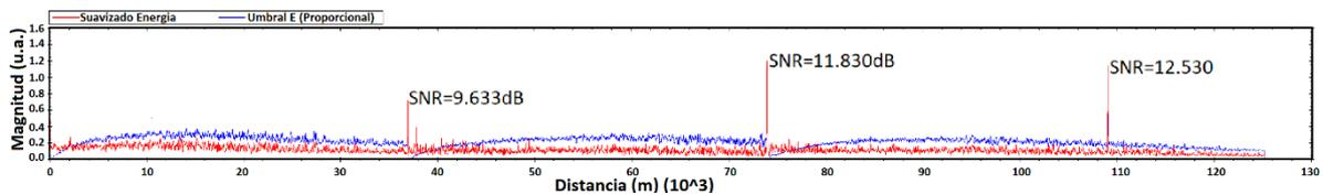
Figure 7: Mechanical vibration (100Hz, 3Vpp) at 37km, 74km and 109km.
