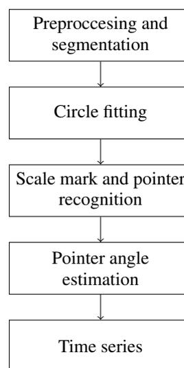
Figure 2: Algorithmic structure of automatic pressure reading system.
