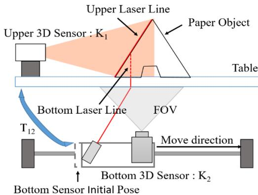
Figure 3: How to scan a calibration object made from one paper with two sensors. We can obtain 3D scanning data of the inner and outer surfaces of calibration objects from two sensors.
