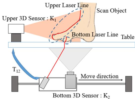
Figure 2: The circular foot scanner consists of an upper 3D scan sensor and a lower 3D scan sensor.
