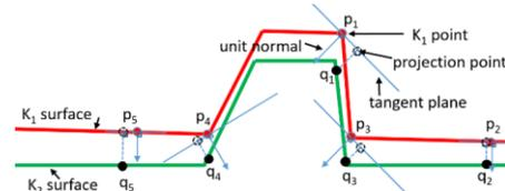
Figure 4: How to use the point-to-plane algorithm to find the transformation matrix between two points.
