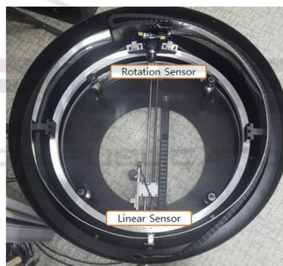
Figure 1: A circular-type 3D foot scanner using structured light sensing method.
