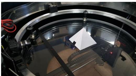
Figure 7: A pyramid object placed at a position visible from both 3D sensors.
