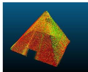
Figure 10: ICP matching result of the two scanned shapes.
