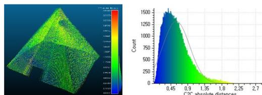
Figure 11: Matching error between the two 3D shapes after ICP transformation.
