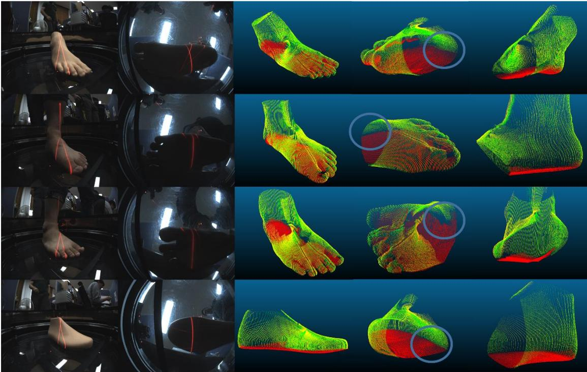
Figure 12: Results of 3D foot models by using the transformation relation between two sensors. From the top, 3D models of a plastic foot model, human left and right foot, and a plastic raster of shoes.
