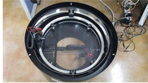
Figure 5: A circular 3D foot scanner for experiments.
