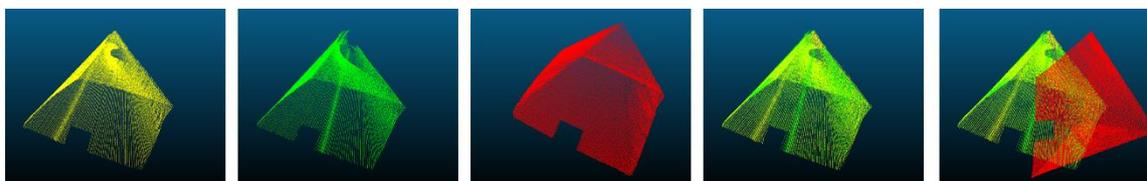
Figure 9: (a) and (b) shows the scanned 3D points of the calibration object using the left and right lasers of the upper 3D sensor, (c) shows the scanned 3D points using lower sensor, (d) shows 3D points that combine (a) and (b), (e) shows two scanned shapes by the upper and lower sensors in the upper sensor's coordinate system.
