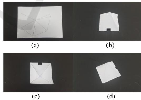
Figure 6: Photographs of the calibration object (a) shows the schematic of the calibration object drawn on a piece of A4 paper, (b) shows outer surface of the object which is scanned by the upper sensor, (c) shows inner surface of the object which is scanned by lower sensors, (d) shows a side view of the calibration object.
