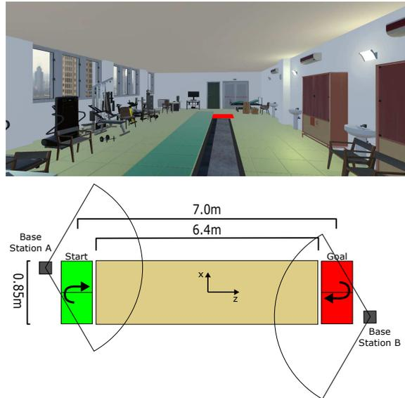
Figure 1: Schematic setup of experiment. (Top) The participants view by wearing the HMD. (Bottom) A sketch of the setup representing the position of the base stations, inversion zones and walkway with the dimensions. The reference system is centered on walkway.
