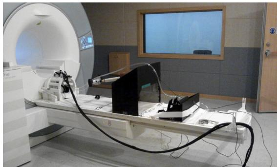
Figure 1: MR-compatible driving system.
