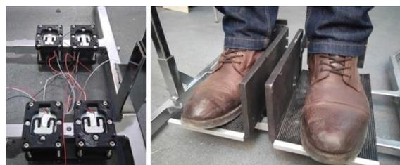
Figure 2: Four YZC-161 load cells bundled to measure weight of the patient (left); standing platforms mounted on the top of the load cells (right).
