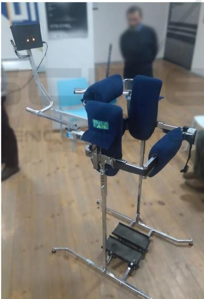
Figure 3: A photograph of the JStep platform with LED display mounted in front of the modified stander.
