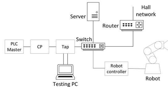
Figure 3: The network structure of our experimental scenario.
