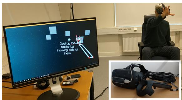
Figure 2: The Ball-throwing level, using the Leap Motion sensor. Inset in the lower-right corner shows the HTC Vive, its controller and the Leap Motion sensor attached to the front of the headset.
