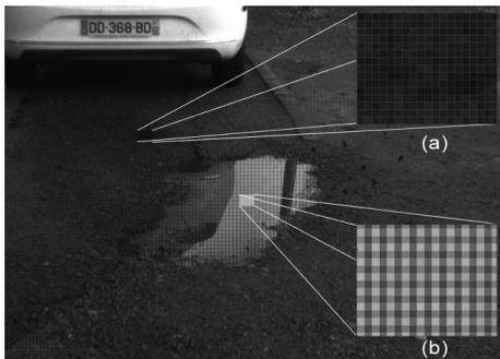
Figure 2: Reflection Influence on Polarimetry. (a) is a zoom on the non-polarized area and (b) on a polarized area. Clearly, on a polarized surface, the micro-grid appears and reveals an intensity change according to the polarizer affected.
