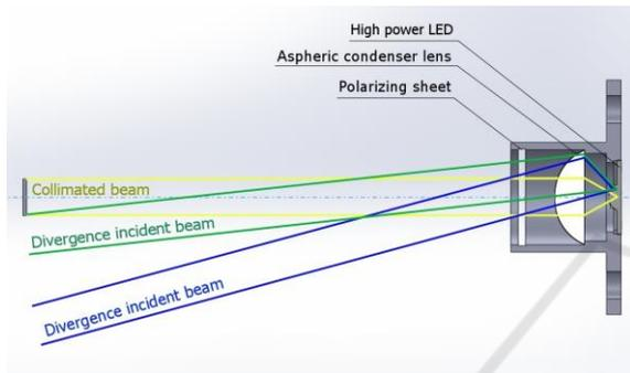
Figure 2: Lighting modules and beam divergence.
