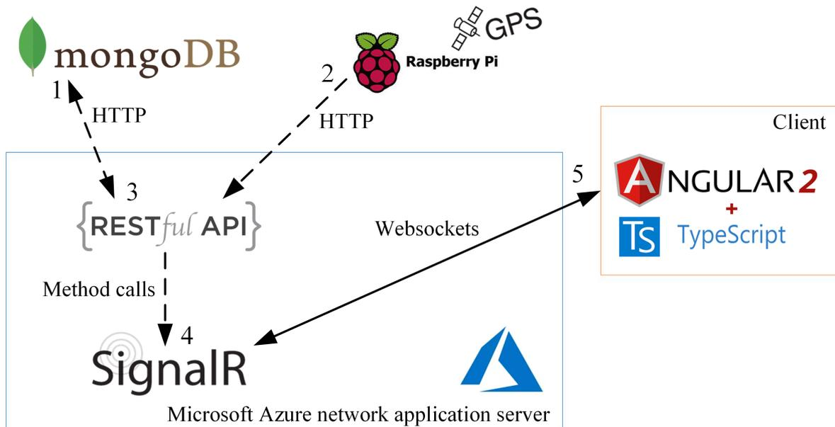
Figure 6: Architecture of the developed system for GPS data visualisation.
