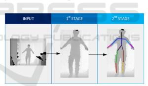
Figure 1: Overview of the proposed top-down YOLO method. The first stage uses a person detector to produce a bounding box around each candidate person. In the second stage, a pose estimator is applied to the image cropped arround each candidate person in order to localize their skeleton's joints.
