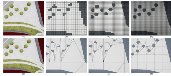
Figure 11: Grid and navmesh representation of the environment. Top row shows three grids with different resolutions: (a) original environment, (b) 128x128, (c) 256x256 and (d) 512x512. Bottom row shows three navmeshes with different voxel size: (e) original environment, (f) 0.5, (g) 0.25 and (h) 0.1.
