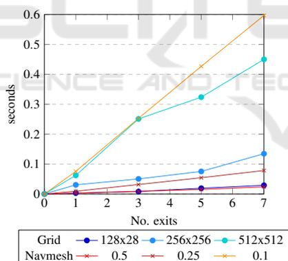
Figure 14: Time taken in seconds to calculate the shortest paths in grids and navmeshes with different sizes.
