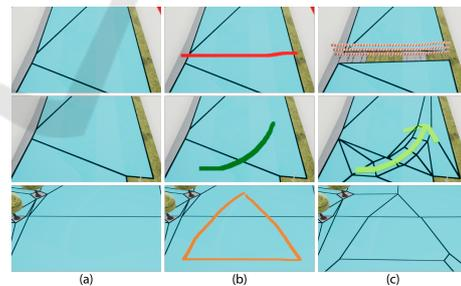
Figure 3: Column (a) original navmesh. Column (b) user-sketched line. Column (c) Updated navmesh with an obstacle (first row), flow line (second row) and area (third row).
