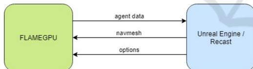
Figure 1: System overview showing the data structures that are exchanged between GPU (green) and CPU (blue).
