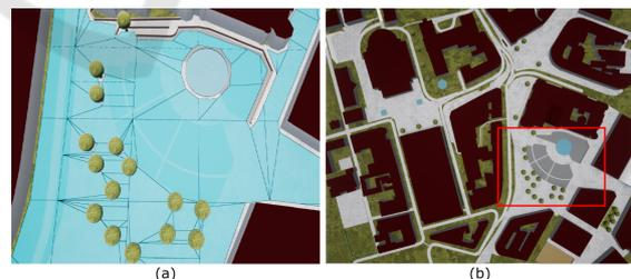
Figure 2: (a) The tiled navmesh created with *Recast* and displayed in *Unreal Engine*. The underlying square tile pattern is shown, as well as the polygons created to connect different parts of the environment such as buildings and trees. (b) The environment where the simulation runs. The red rectangle highlights the area shown in (a).
