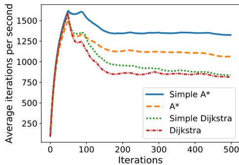
Figure 5: Performance comparison of path planning algorithms with and without the assumed simplification.
