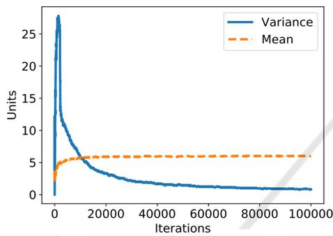
Figure 4: Mean and variance of all actual edge lengths over more than 100,000 iterations of NGDPP.
