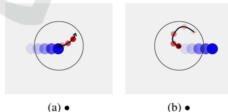
Figure 3: An agent (red) evades a collision object (blue) within its force field. After the collision object leaves the detection radius, the agent returns to the center.
