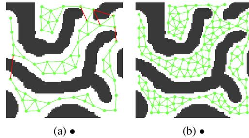
Figure 1: In the comparison of the SGNG with low (a) and high precision (b), it is noticeable that in the first case wrong (not collision-free) edges can be formed (colored in red).
