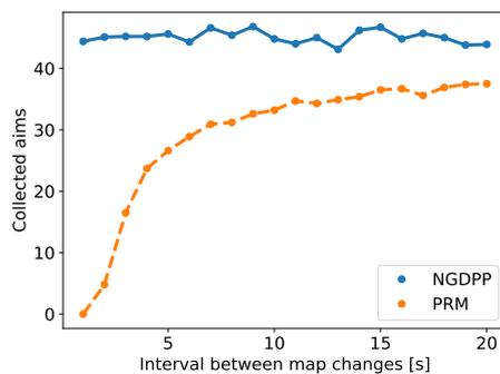
Figure 9: Performance comparison of NGDPP to a simple PRM implementation (adapted from (Sakai et al., 2018)).
