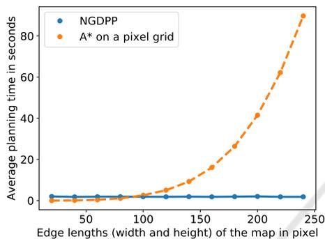
Figure 8: Performance comparison of NGDPP to A\* routing on a graph that results from interpreting every pixel of the input floor plan as node.
