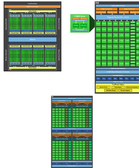
Figure 3: Processing units packaging within a GPU.
