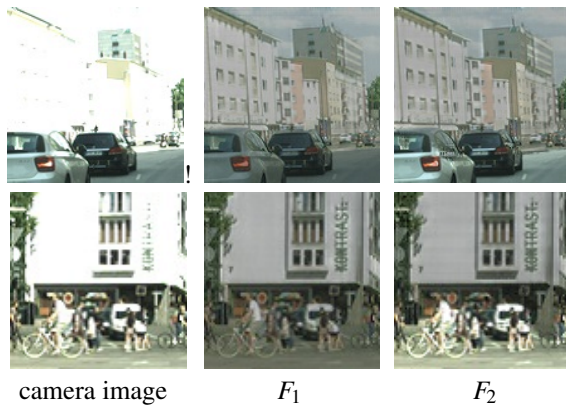
Figure 9: Comparison of the tone mapping functions, F_1 and F_2 , used in the training step of our network. Both F_1 and F_2 enable us to see faraway buildings and their details, which are not visible in the original camera images. However, the visibility of pedestrians is degraded in F_1 , while that is preserved in F_2 .
