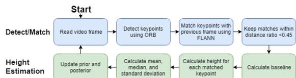
Figure 4: An overview of the program used to estimate the free height of the drone.
