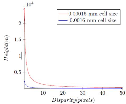
Figure 2: The estimated height plotted as a function of displacement in pixels using the hypothetical values; 20mm focal length and 100mm baseline. Although pixels are discrete values, they have been plotted as continuous for readability.
