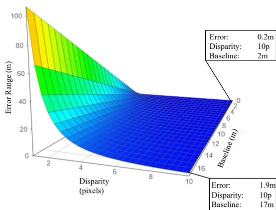
Figure 3: Relationship between disparity and baseline on single pixel error.
