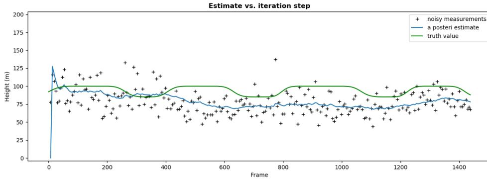
Figure 8: The estimated heights at a varying 100m free height before and after filtering.
