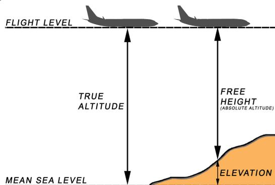
Figure 1: Figure illustrating the free height of a drone.
