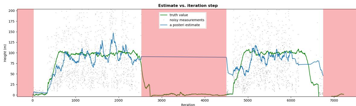
Figure 10: Ground truth, raw measurements and filtered results. Red areas represents data not included in the calculations as the drone is not flying or no data was recorded.
