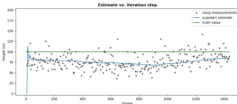
Figure 6: The estimated simulated heights at a constant 100m free height before and after filtering.
