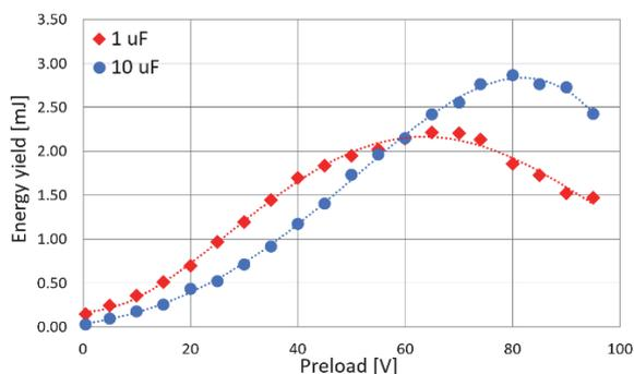
Figure 4: Energy yield of piezo buzzers at different preloads and with two different storage capacitor sizes.
