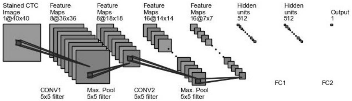
Figure 5: The ConvNet Architecture.
