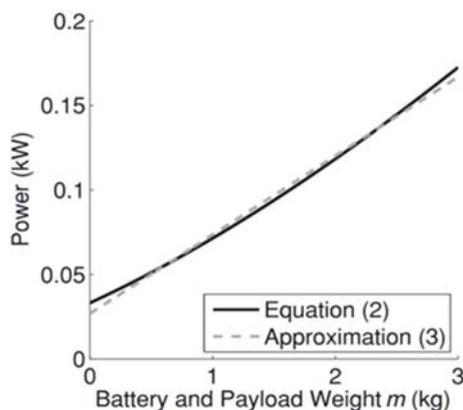
Figure 1: Power pattern in an hexacopter UAV, approximately linear with the total load on board (Source: (Dorling et al.,2017)).
