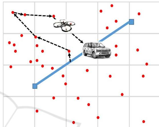
Figure 2: Target Scenario: UAV and GV moves separately. The dashed lines represent fly paths for UAV.
