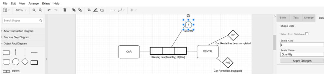
Figure 4: OFD drawn using the DISME Diagram Editor.
