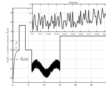
Figure 8: Uncertainty  $D_d(2) = f$  (dotted line) as shown in Fig. 1 and its estimate  $\hat{D}_d(2)$  (solid line).
