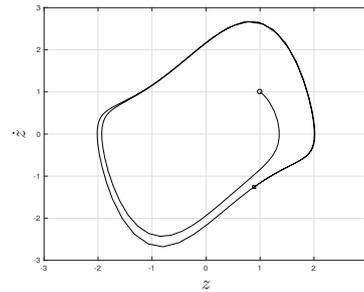
Figure 2:  $z - \dot{z}$  phase plane with  $u = 0$  and  $f = 0$ .
