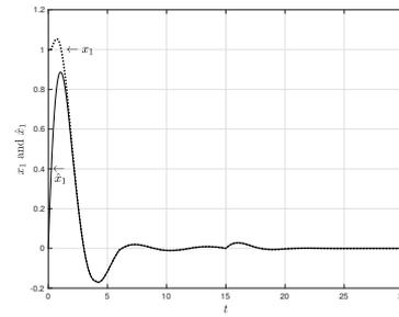
Figure 5: State  $x_1$  and its estimate  $\hat{x}_1$  driven by the proposed controller (41) along with the observer (4) where the uncertainty in (54) is applied.
