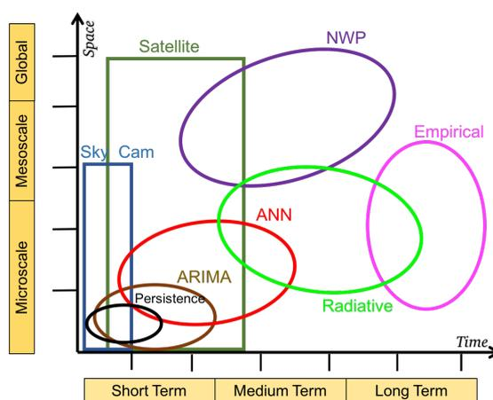
Figure 1: Spatial and temporal domains of solar irradiance models, adapted partly from (Pelland et al., 2013; Diagne et al., 2013).
