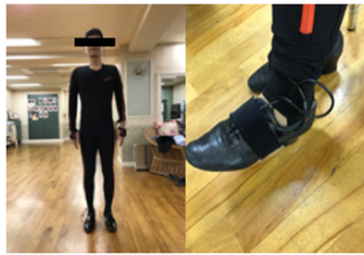
Figure 1: The IMUs were set with a purpose-build suit (left). The IMU was strapped over a shoe (right).
