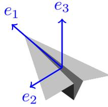
Figure 3: Body coordinate system (Paiva and Fontes, 2018).
