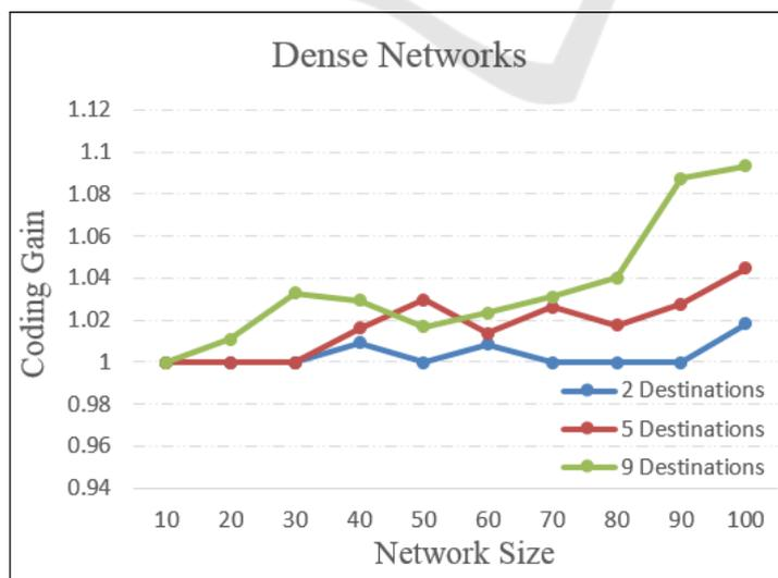
Figure 11: Coding Gain in Networks of High Density.
