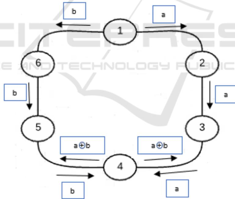
Figure 5: Packet Transmission using NC.
