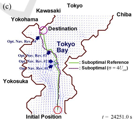
Figure 8: Monitored vehicle trajectories by suboptimal navigation in a tidal flow in Tokyo Bay observed at (a) 12000.0 s (b) 18000.0 s (c) 24251.0 s.
