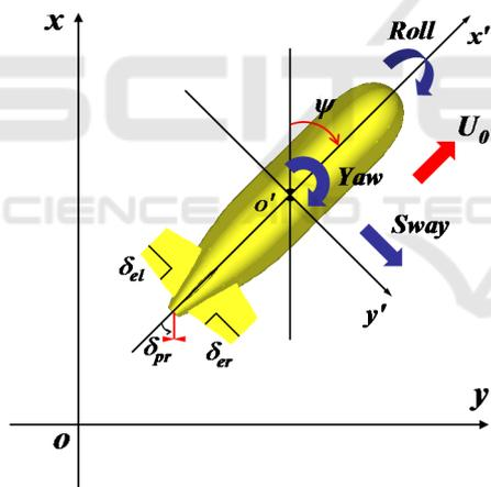
Figure 1: Coordinate systems for optimal guidance problem formulation.
