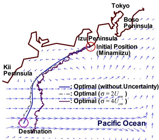
Figure 6: Vehicle trajectories in a Northwestern Pacific Ocean region. In this example, on-site sea current velocities are generated to include uncertainties expressed by AWGNs.
