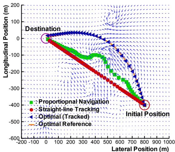
Figure 3: Vehicle trajectories in a vortical source flow.
