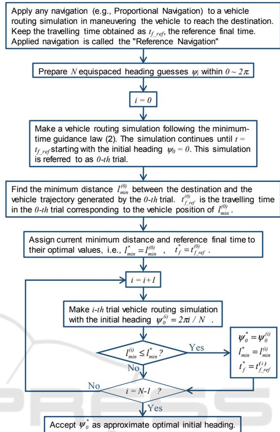
Figure 2: Algorithmic scheme of the numerical solution procedure AREN for deriving the optimal initial heading.
